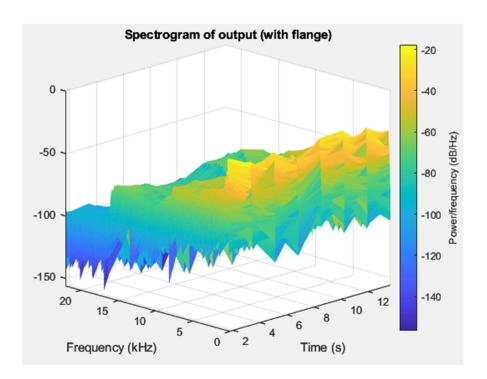
Pictured above are the spectrograms of the unflanged input and the flanged output. This time, the difference between the input and output are more noticeable than they were in the FFT chart, as the negative power spectral spikes due to the interference pattern are visible in the second plot, while in the first plot they are much smaller in number and in amplitude.
