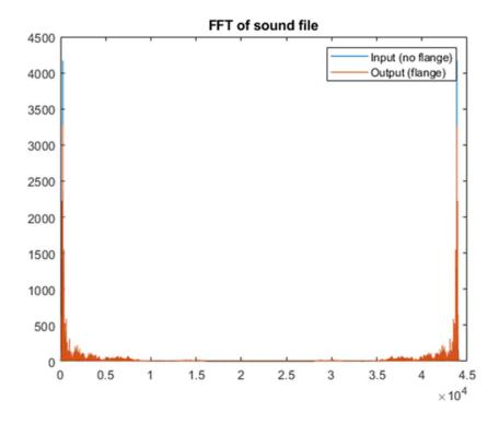
Pictured above are the Fast Fourier Transforms of both the unflanged input and the flanged output. While there is not a large amount of difference, we can see that there is at least some cancellation of the very large spectrum peaks caused by the interference pattern from the flange signal combination process.
