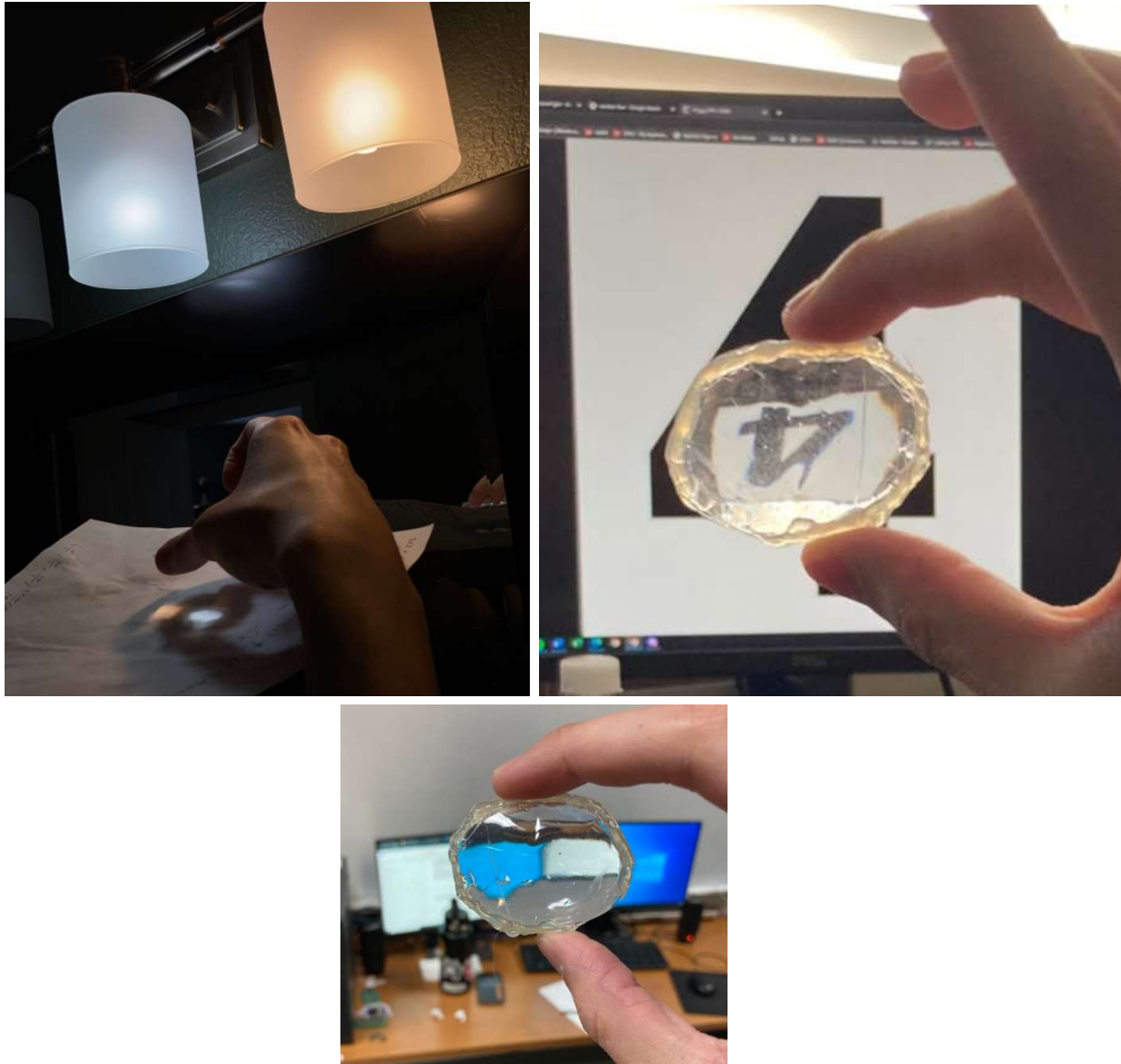
Fig 3: Inversion of bulbs (left), inversion of screens (middle), inversion of the number 4 (right)
