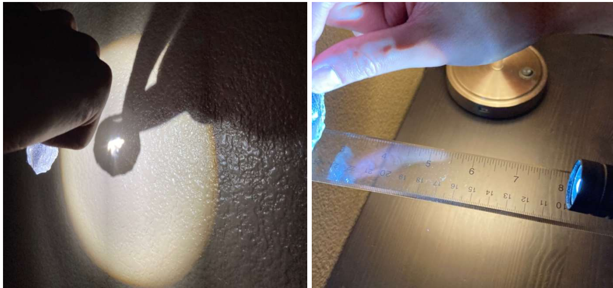
Fig 2: Focal point showing converging of light (left), distance between light, lens, and screen (right)
