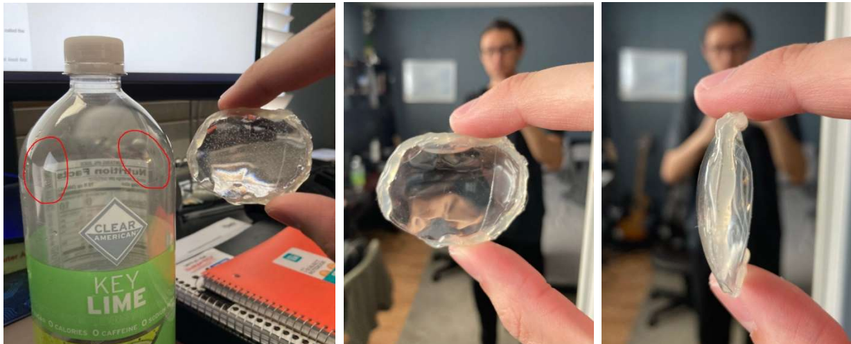
Fig 1: Bottle used (left), finished lens from the front (middle), finished lens from the side (right)
